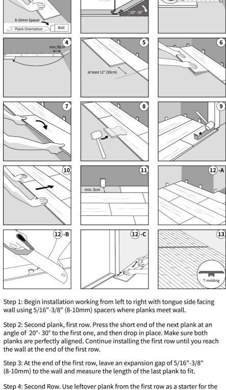
second row. To achieve a better effect, the small plank should measure at least 12" (30cm). Otherwise, cut a new plank in half and use it to begin the second row. Whenever practical, use the piece cut from the preceding row to start the next row.
