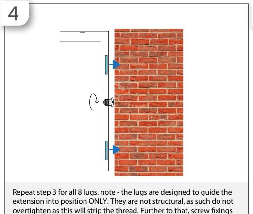
directly into the aparture are required to hold the door in position.
