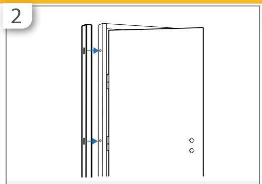
Screw in the window out lugs into the extension & slow over the side of your door. Repeat on both sides if necesary.
