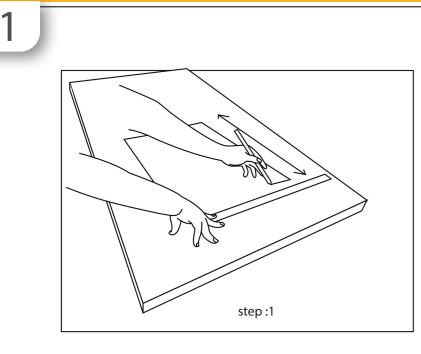
Lay door on a flat stable surface taking care not to scratch or damage the door. Mark out the cut with a pencil in the desired position using a straight edge & pencil. Note, 150mm clearance must be left around all 4 sides of the door. You can use the internal measurement of the vent/window frame as a template to draw around.
