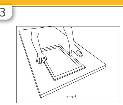
Insert window or louvre vent frame on both sides and check snug fit. If need to recut accordingly. Once satisfied with the aperture, begin if the EXTERNAL FACE first.
