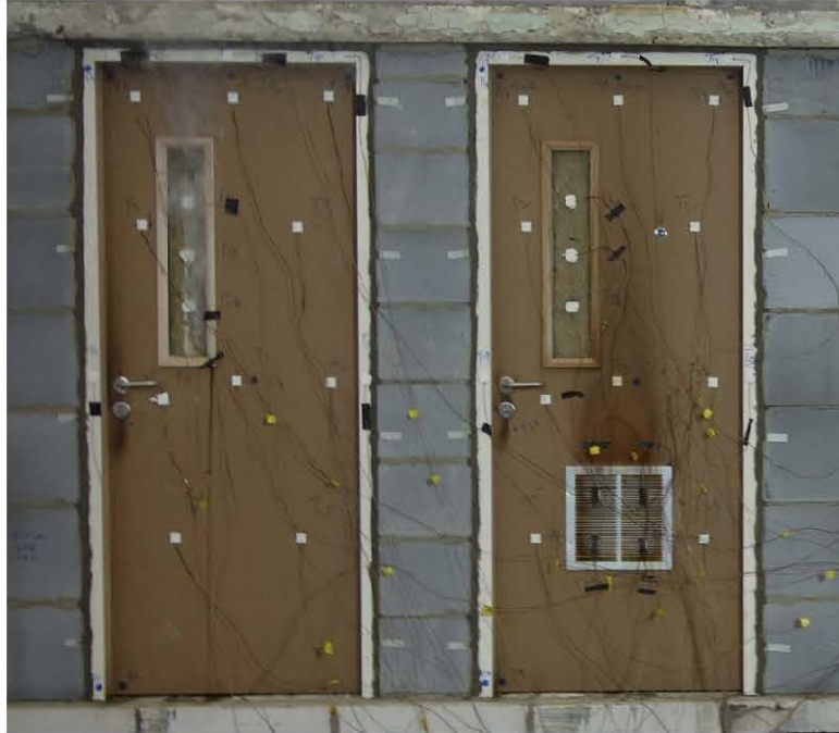
Fig. 3 Unexposed Side after 10 Minutes
