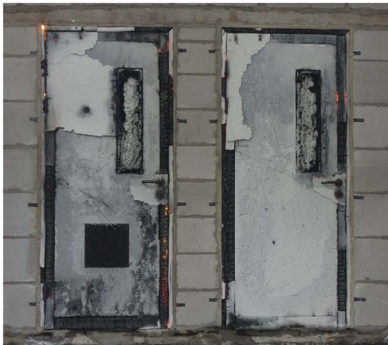
Fig. 8 Exposed Side after 68 Minutes
