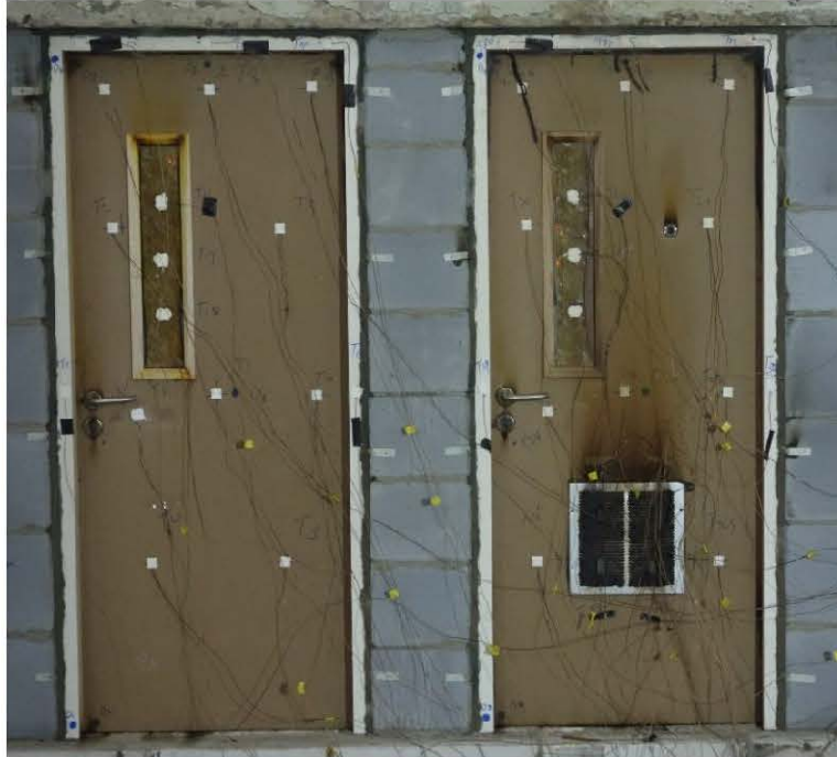
Fig. 7 Unexposed Side after 68 Minutes
