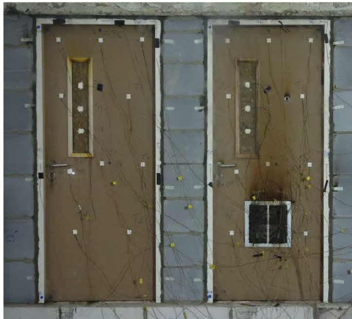
Fig. 6 Unexposed Side after 60 Minutes
