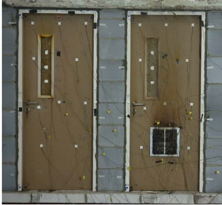
Fig. 5 Unexposed Side after 50 Minutes
