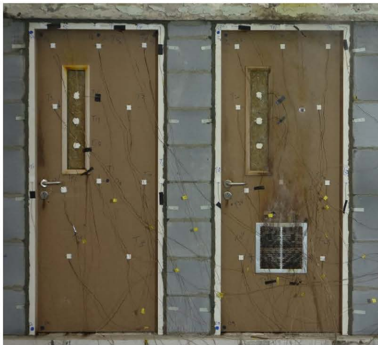
Fig. 4 Unexposed Side after 30 Minutes
