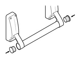
Test several times by closing and fully engaging the push pad to release. Apply vinyl signage as necessary (sold separately).
