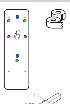
To fit Push Pad/Bar lever, cut the spindle to 67mm. Insert into place & place over template on the Exterior of the door. Ensure level/square & apply masking tape to secure.
