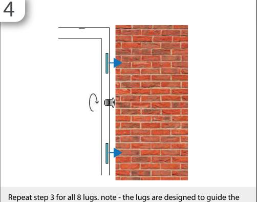
extension into position ONLY. They are not structural, as such do not overtighten as this will strip the thread. Further to that, screw fixings directly into the aparture are required to hold the door in position.
