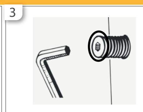
Hold the side panels in position & insert the door into the aparture. Prop the door in position (2nd person may be required), open the door and locate the wind out lugs through the tabs on the inside of the frame. Using a hex key, wind in or out the lugs until the frame extension sites tight against the aparture. DO NOT OVERTIGHTEN.
