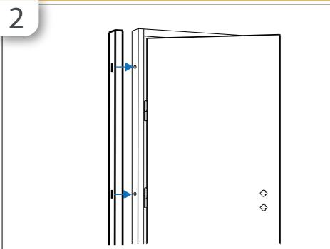
Screw in the window out lugs into the extension & slow over the side of your door. Repeat on both sides if necesary.
