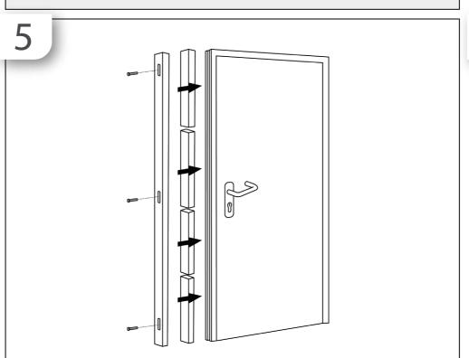
After you have the expansion panels set at the correct distance, remove the door and fill the gaps with rockwool insulation provided. Pack tighlty for best results.
