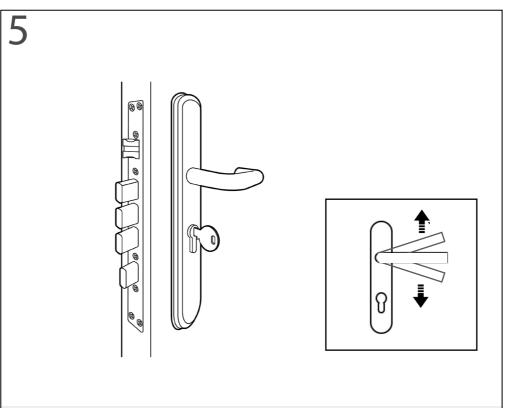
Test the key lock to finish. Note the door features quick lift-to-lock function and can be locked by lifting the handle upwards from the external side.
