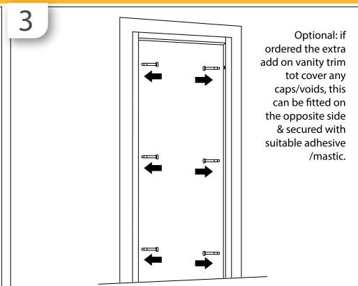
Use anchor bolts or suitable frame fixings to secure in place (washers are advised). NOTE - due to various types of frame being installed into ie. brick, metal, timber
