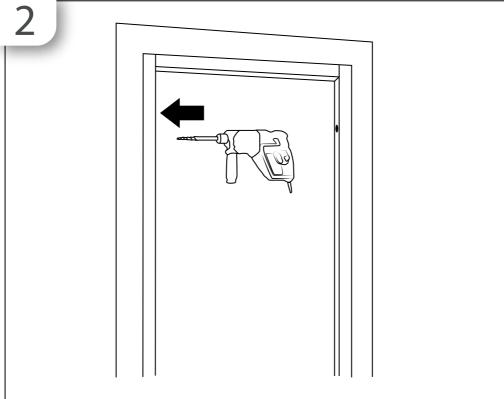
Once door is square & firmly in position, using the pre-drilled tabs, mark fixing positions on the building lining/frame & drill using suitable drill bit.
