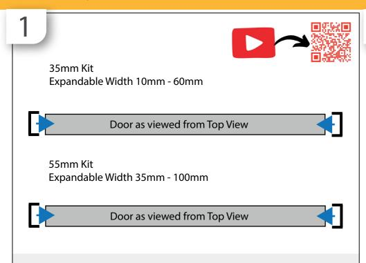
Our standard door widths are 840mm / 940mm / 1040mm. If you need a door with inbetween these, we have extension side infill panels. Simply select which size of kit you require:
