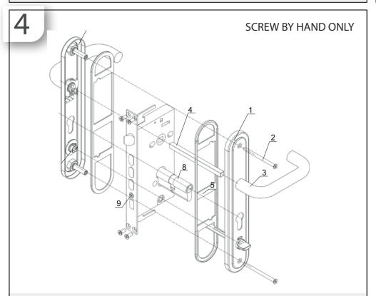
Install the handle by securing with the 2 screws from the inside. Note the eurocylinder isnt centre 90mm(50/40) - the longest end faces external as well as the spindle which is in 2 halves to allow for lift-to-lock function.
