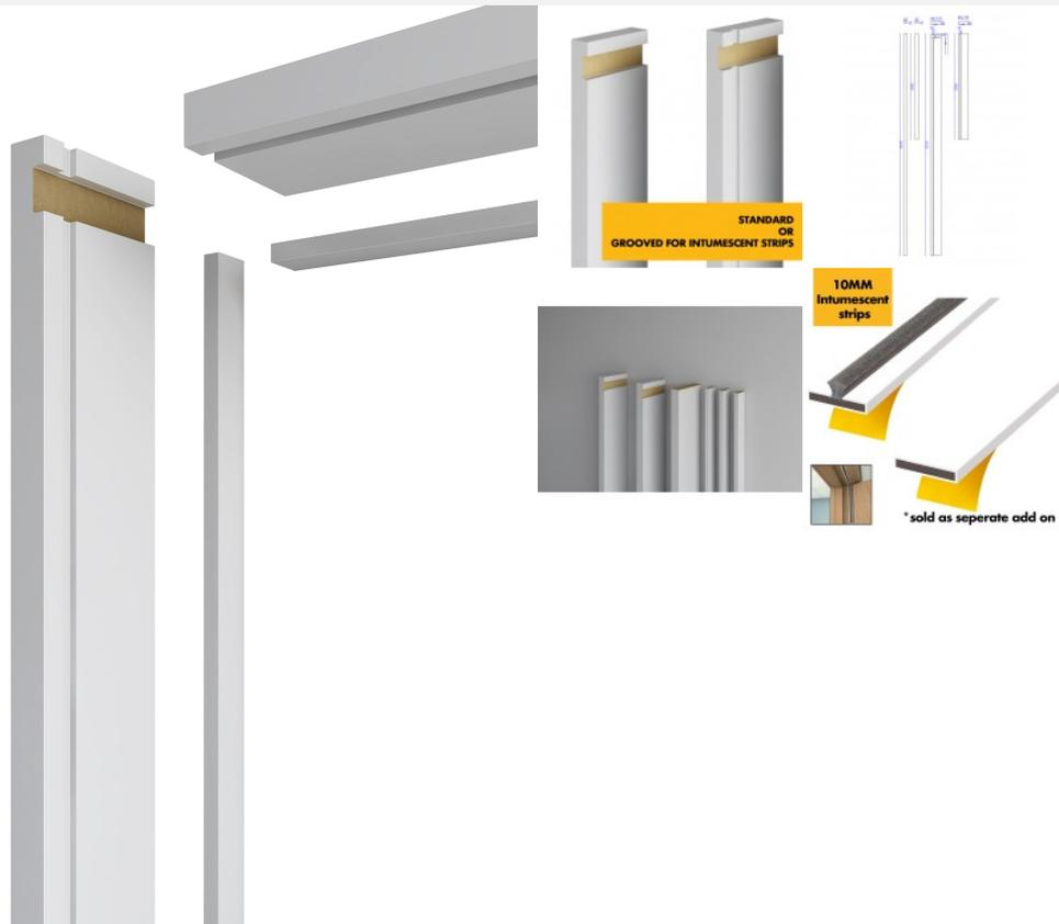
**Universal width - kit comes with 1000mm wide header that can be cut to fit any door sizes such as 680mm, 762mm, 840mm etc. Legs are notched to support single piece header which is universal and can be cut to fit any width of door.**
